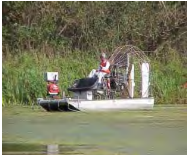
Airboat equipped for liquid and pellet herbicide applications
