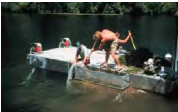
Diver assisted dredge being tested at Wakulla Springs. Above, diver operating suction dredge; right, hydrilla filling catch basket on barge; below, two dredge units in operation to increase efficiency.
