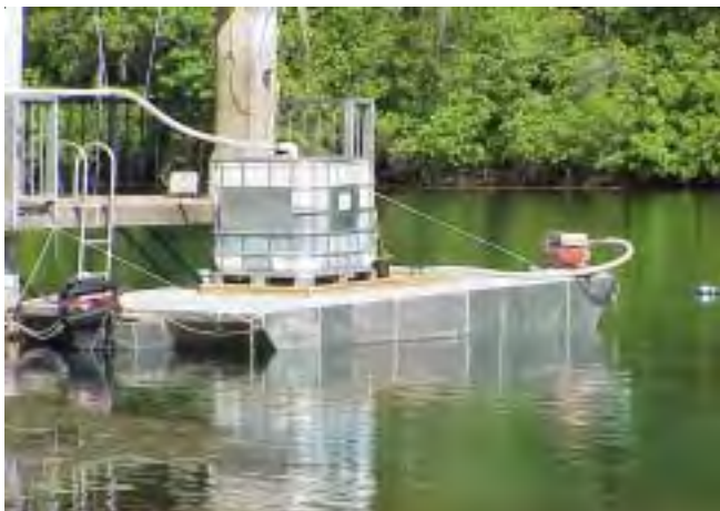
Metering endothall herbicide into the headwaters of the Wakulla River for downstream hydrilla control
