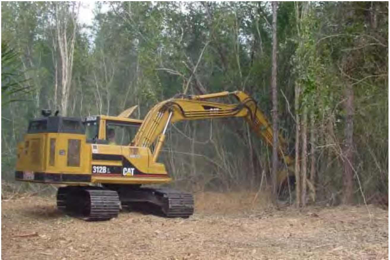
The powerful cutting head of the Brontosaurus reduces entire trees to mulch.
