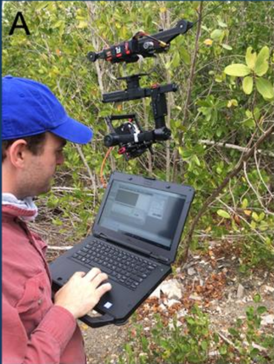
Photos. A-Setting up the flyine and hyperspectral camera and, B-conducting a pass to collect data from a site off of the Rowdy Bend Trail in Everglades National Park.
