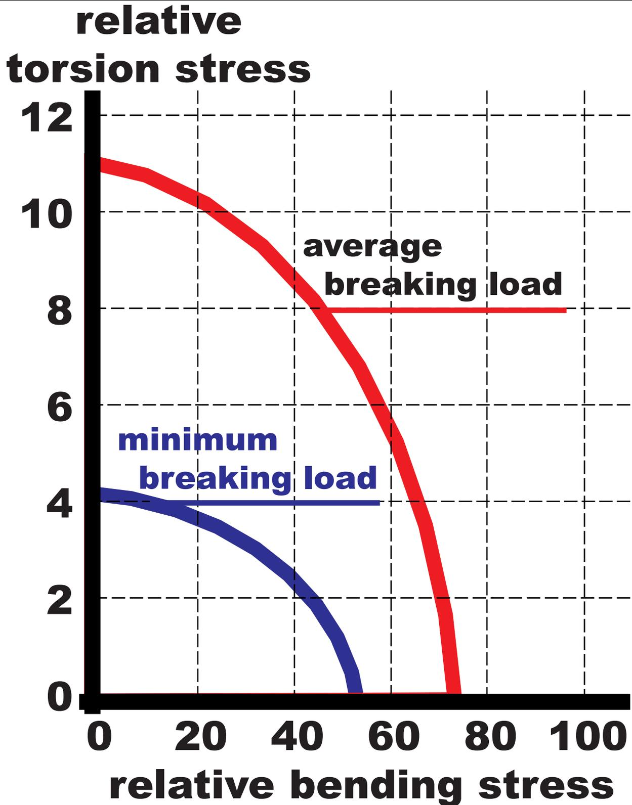
Figure 19: Relationship between relative bending and torsion loads in breaking branches. (Avalos & Sanchez 2014)
