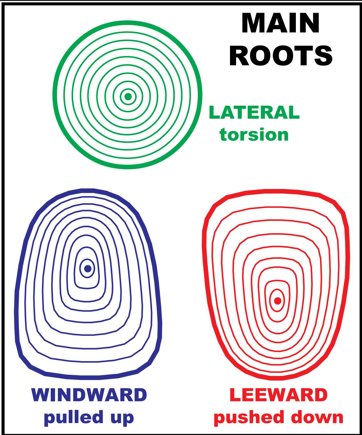
Figure 29: Eccentric growth form of structural roots generated around a tree base to resist wind induced loads. (Stubbs et al. 2019)
