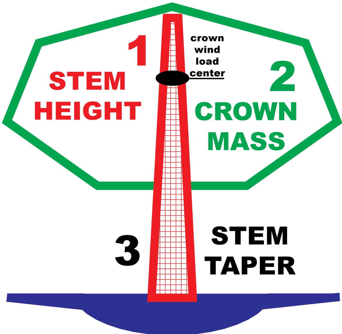
Figure 14: Height related structural components in trees optimized to maintain a tree upright against gravity and wind loads.
