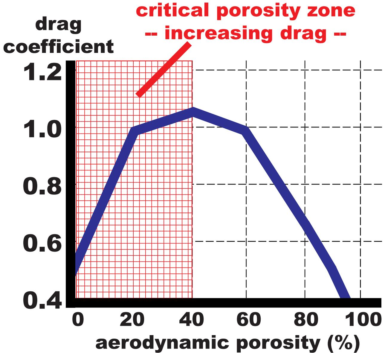
Figure 11: Comparing aerodynamic porosity of tree crowns and tree drag coefficients. (Manickathan et al. 2018)
