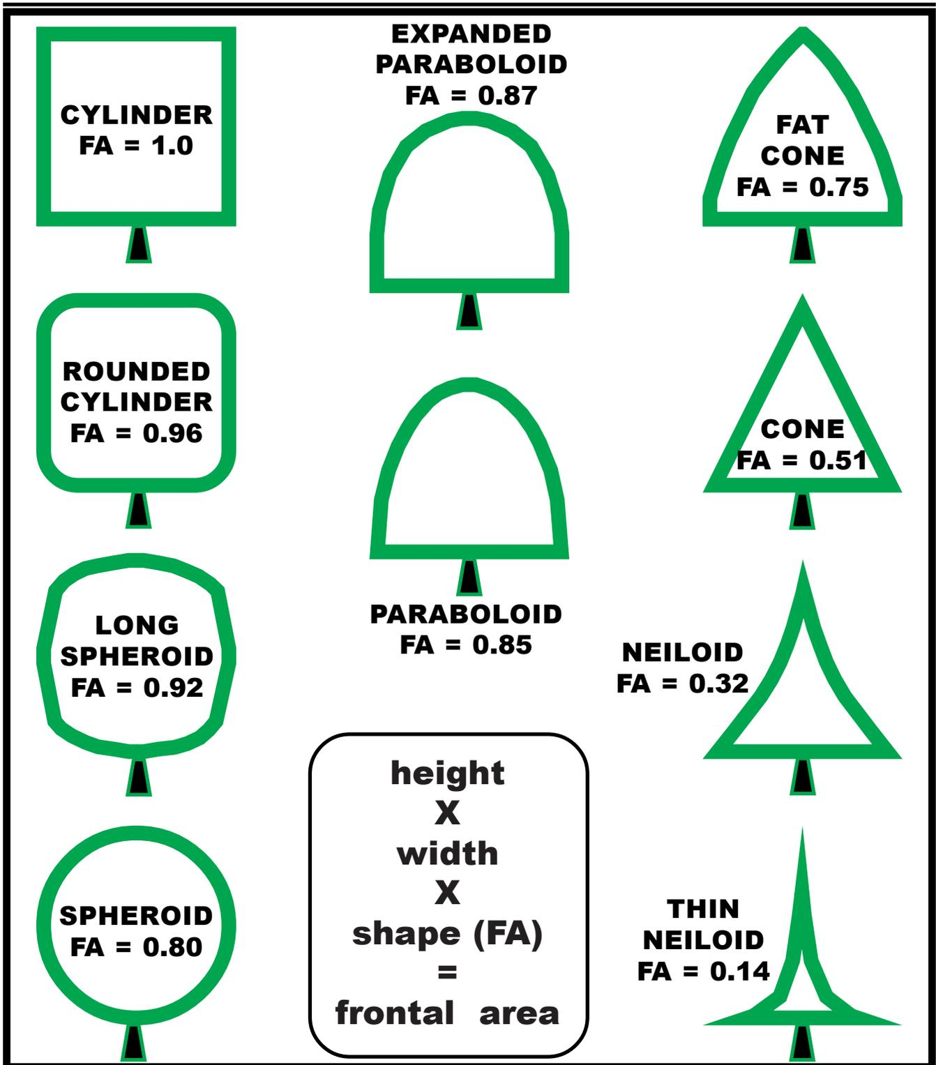
Figure 5: Primary geometric tree crown shapes with relative frontal areas (FA) given under no wind load.
