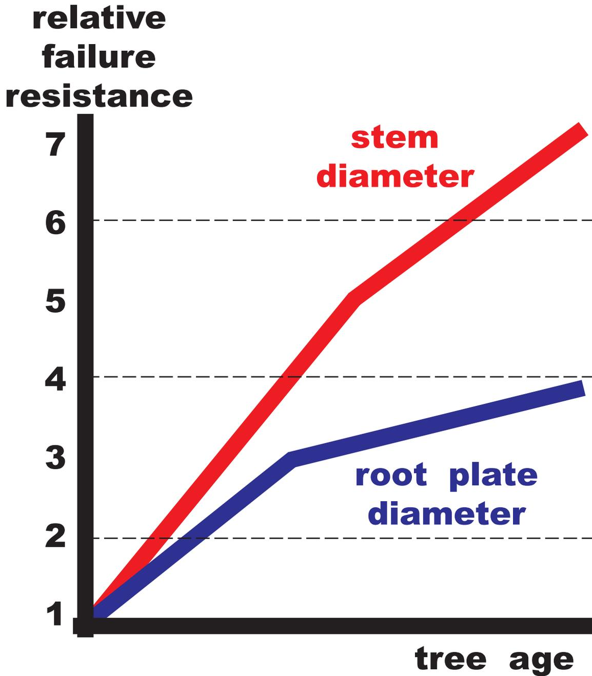
Figure 34: Change in relative resistance to failure of root plate diameter and stem diameter as trees age.
