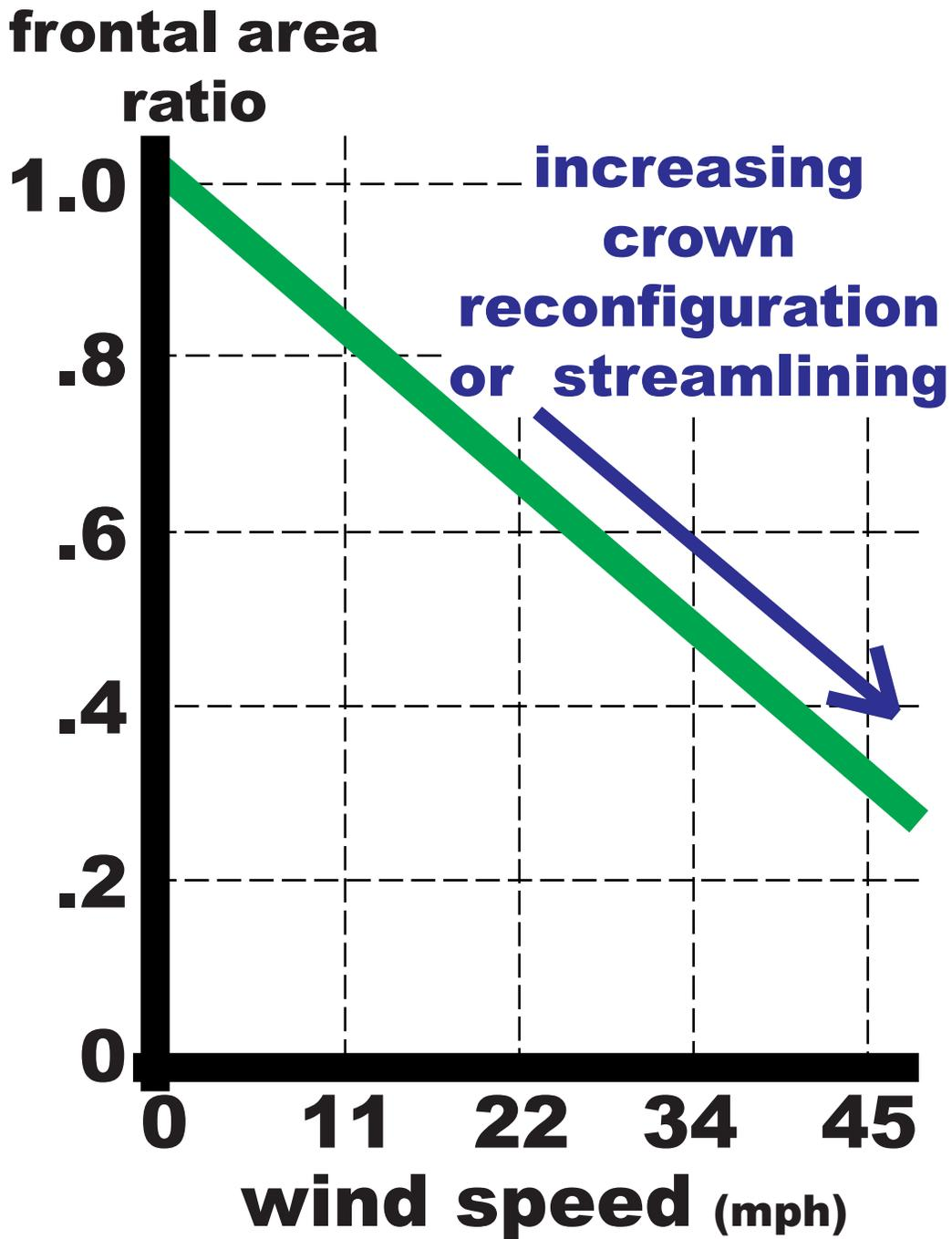
Figure 8: Frontal area ratio (frontal area / still-air frontal area) for unpruned hardwoods versus wind speed. (after Vollsinger et al. 2005)
