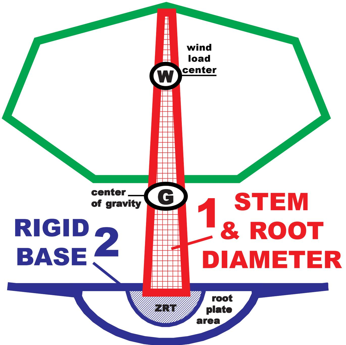
Figure 23: Diameter related structural components optimized to maintain a tree upright against gravity and wind loads.
