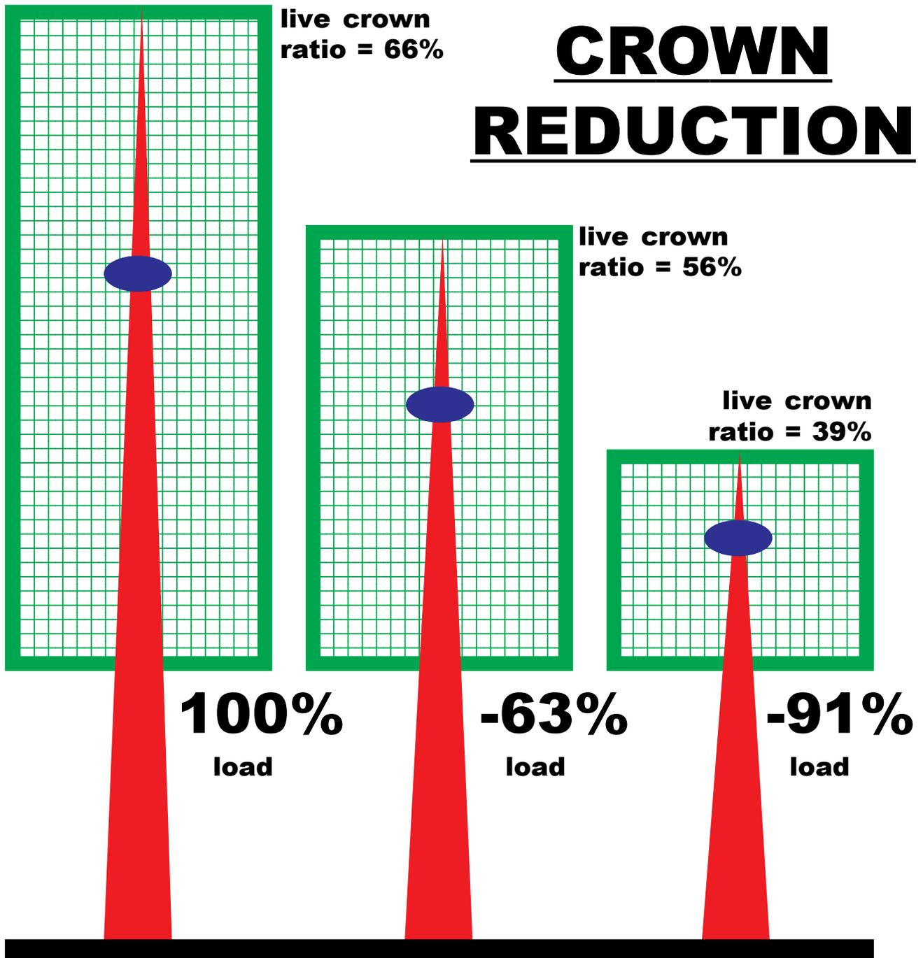
Figure 22: Relative tree wind load decreases under two crown reduction treatments (1/3 & 2/3). The blue oval is the crown wind load center.
