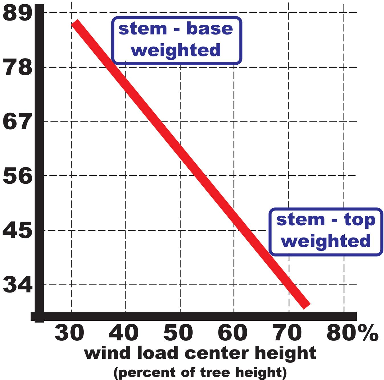
Figure 15: Example tree failure wind speeds versus tree wind load center's height. (after Urata et al. 2012)
