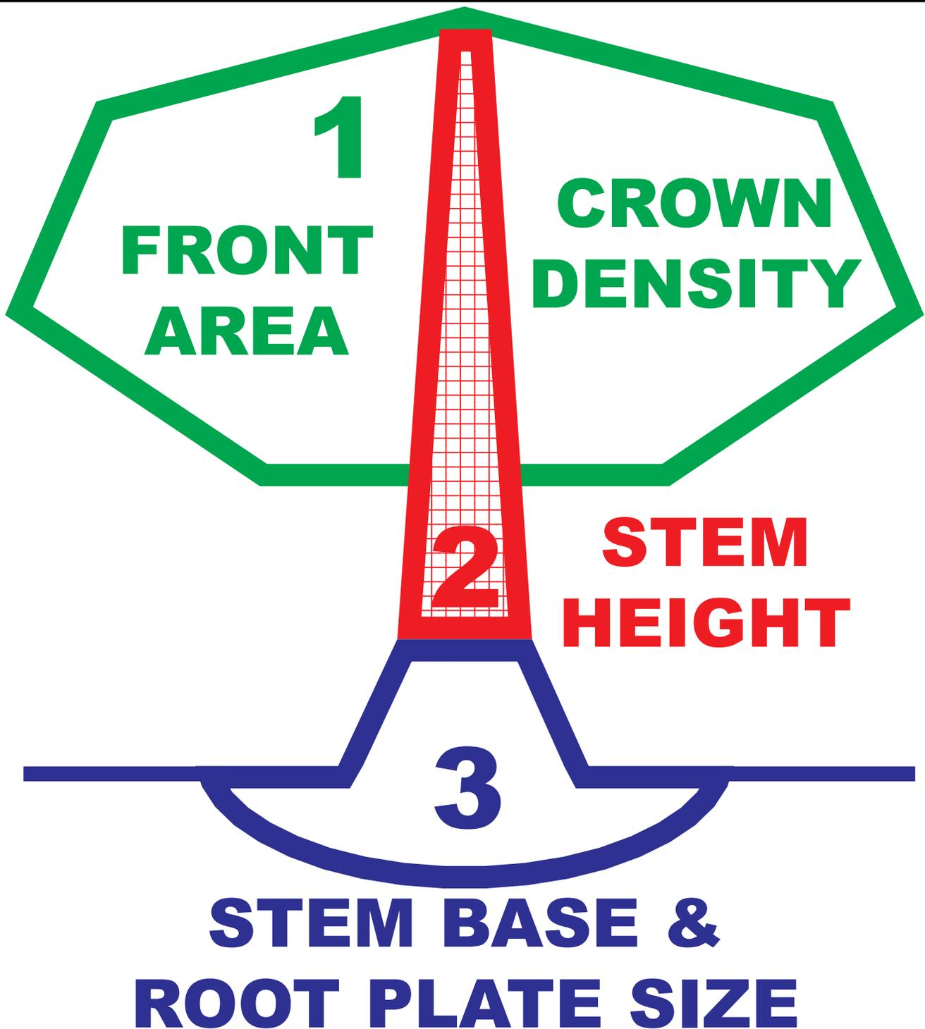
Figure 1: Three primary structural components in trees (sail, height, size) optimized to maintain a tree upright against gravity and wind induced loads.
