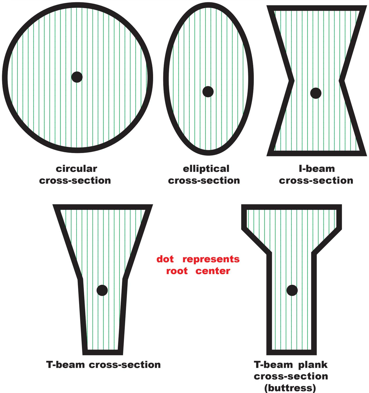
Figure 30: Idealized shapes of root base cross-sections as diameter growth responds to mechanical stress.
