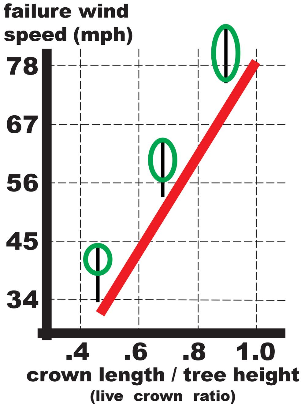
Figure 18: Failure wind speed for a tree versus its crown length / tree height (live crown ratio).
