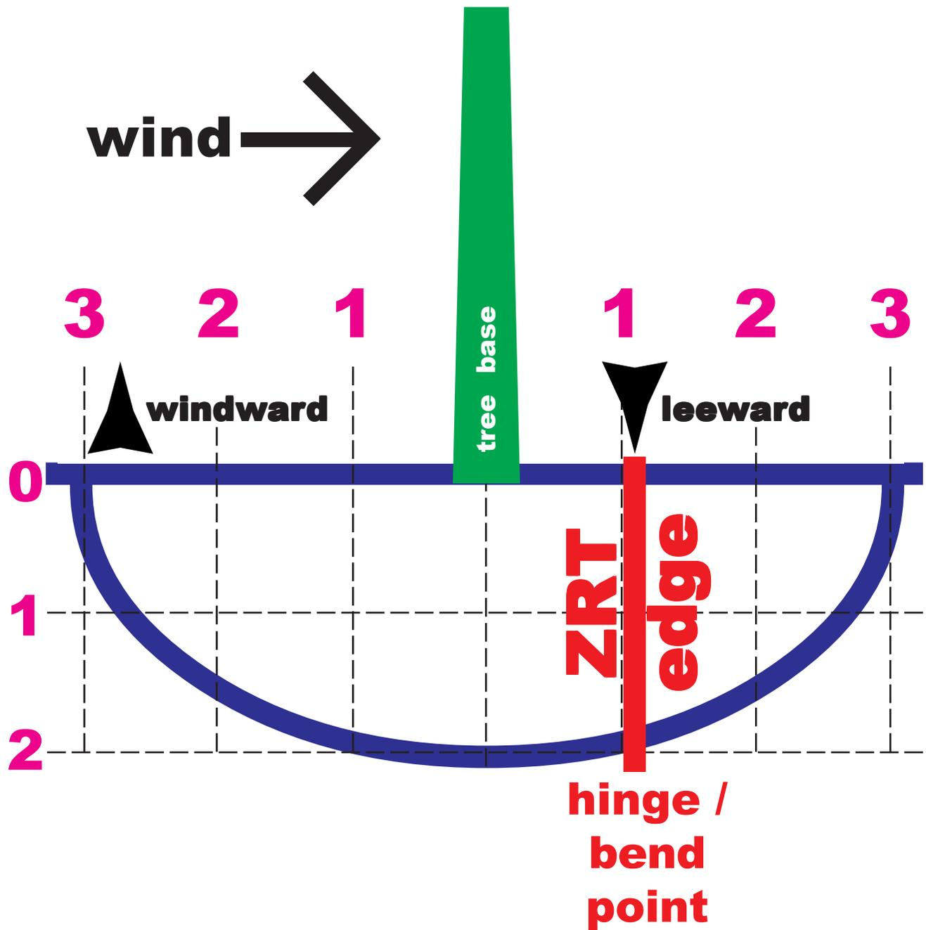
Figure 32: Idealized side view of a wind loaded root plate and edge of ZRT under non-limiting soil conditions. (Coder 2010; Coder 2018; Danjon et al. 2005; Lundstrom et al. 2007)
