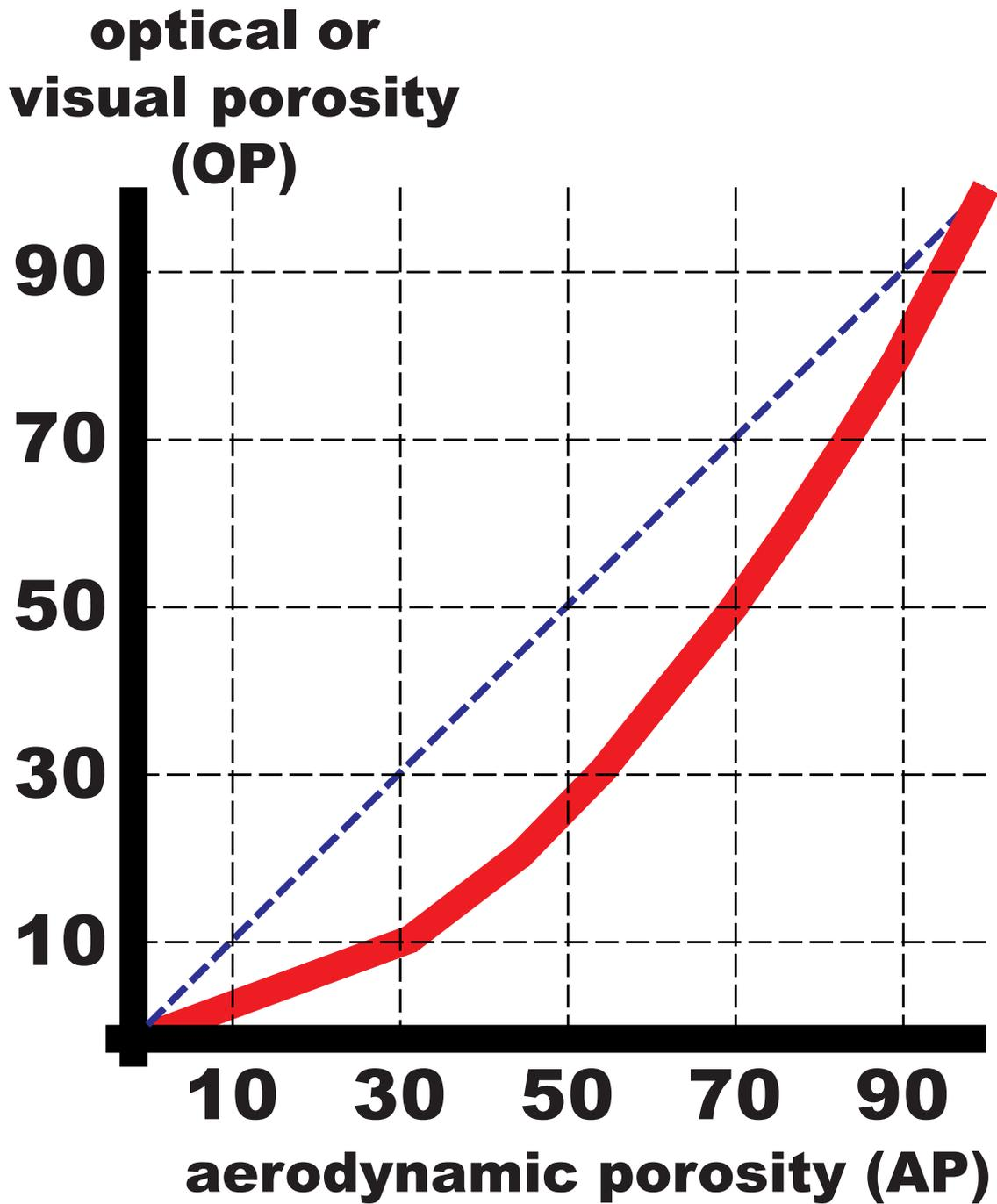
Figure 10: Comparing visual or optical crown porosity (OP) with aerodynamic crown porosity (AP).
