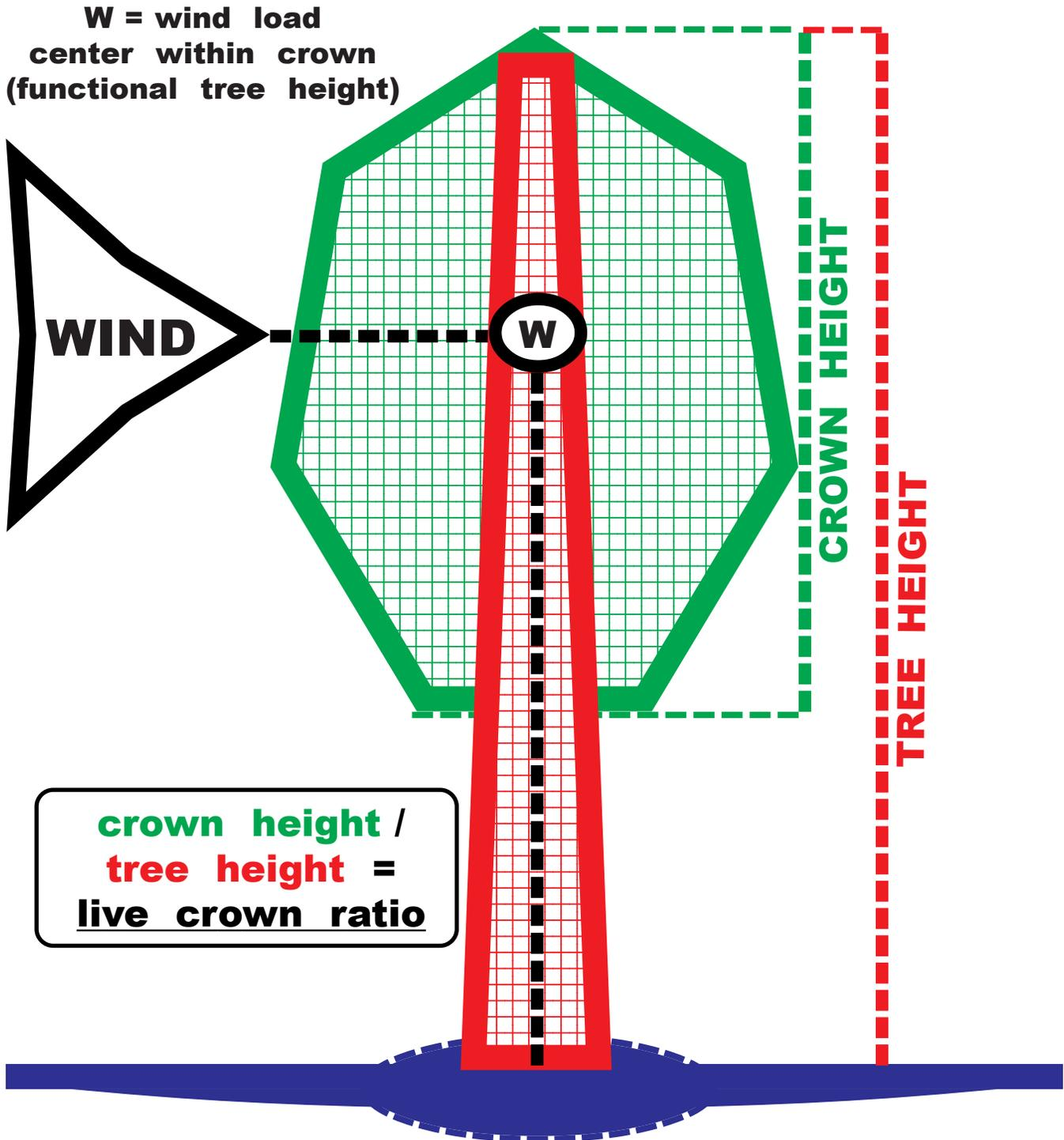
Figure 16: Tree structural model showing total tree height, functional tree height (height of wind load center in crown), and live crown ratio.
