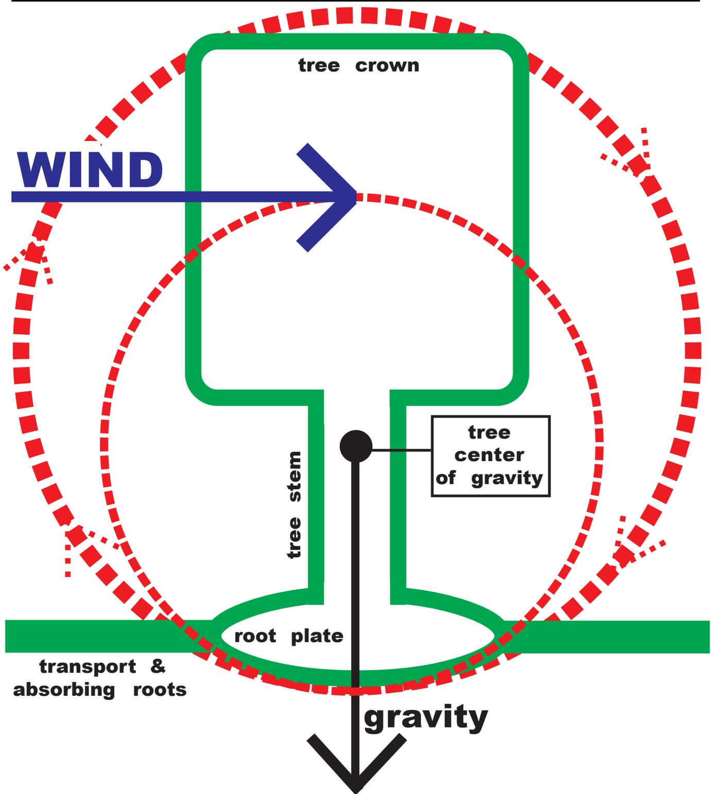
Figure 27: Simplified view of wind and gravity loads acting to rotate a tree out of soil as a combined load wheel.
