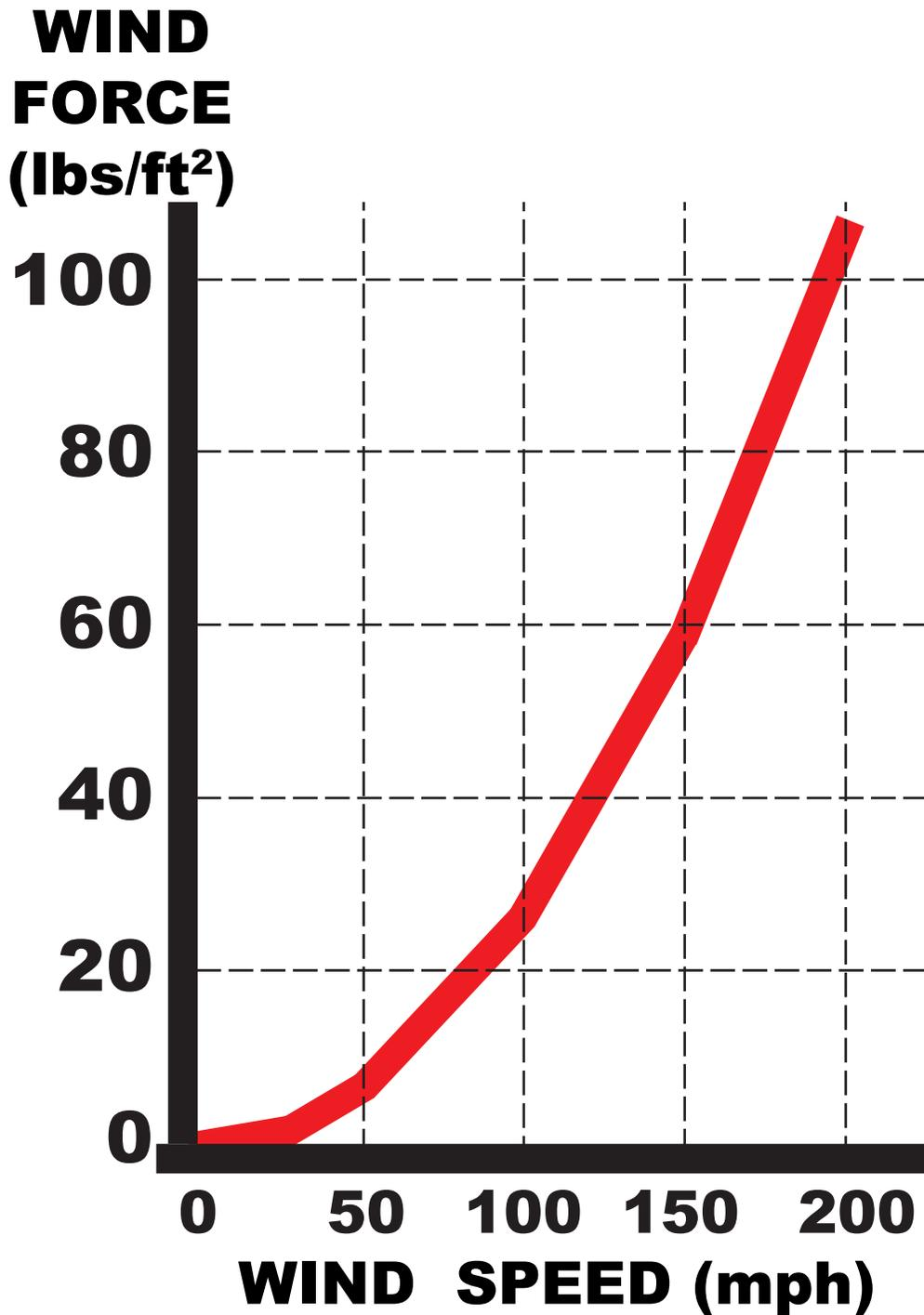
Figure 3: Estimated pressure or force of wind at different wind speeds applied to frontal area of trees. (drag coefficient = 1.0)
