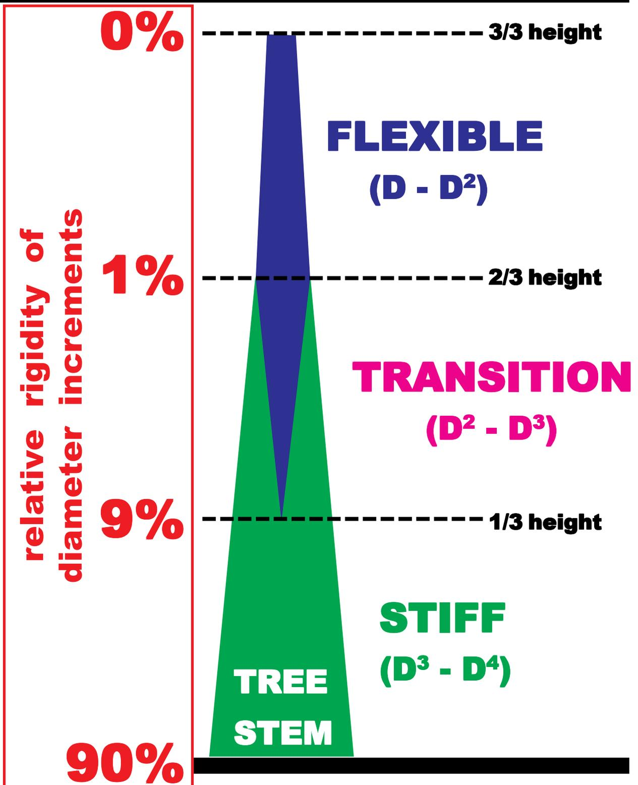
Figure 26: Tree stem stiffness and flexibility zones based upon calculated diameter increment values ( $D^x$ ) and comparative rigidity of diameter increments at each location.
