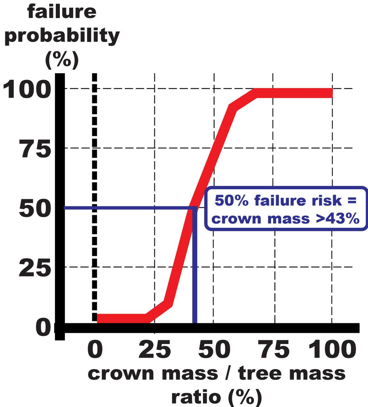
Figure 20: Probability of tree failure based upon crown mass proportion of above-ground tree mass.
