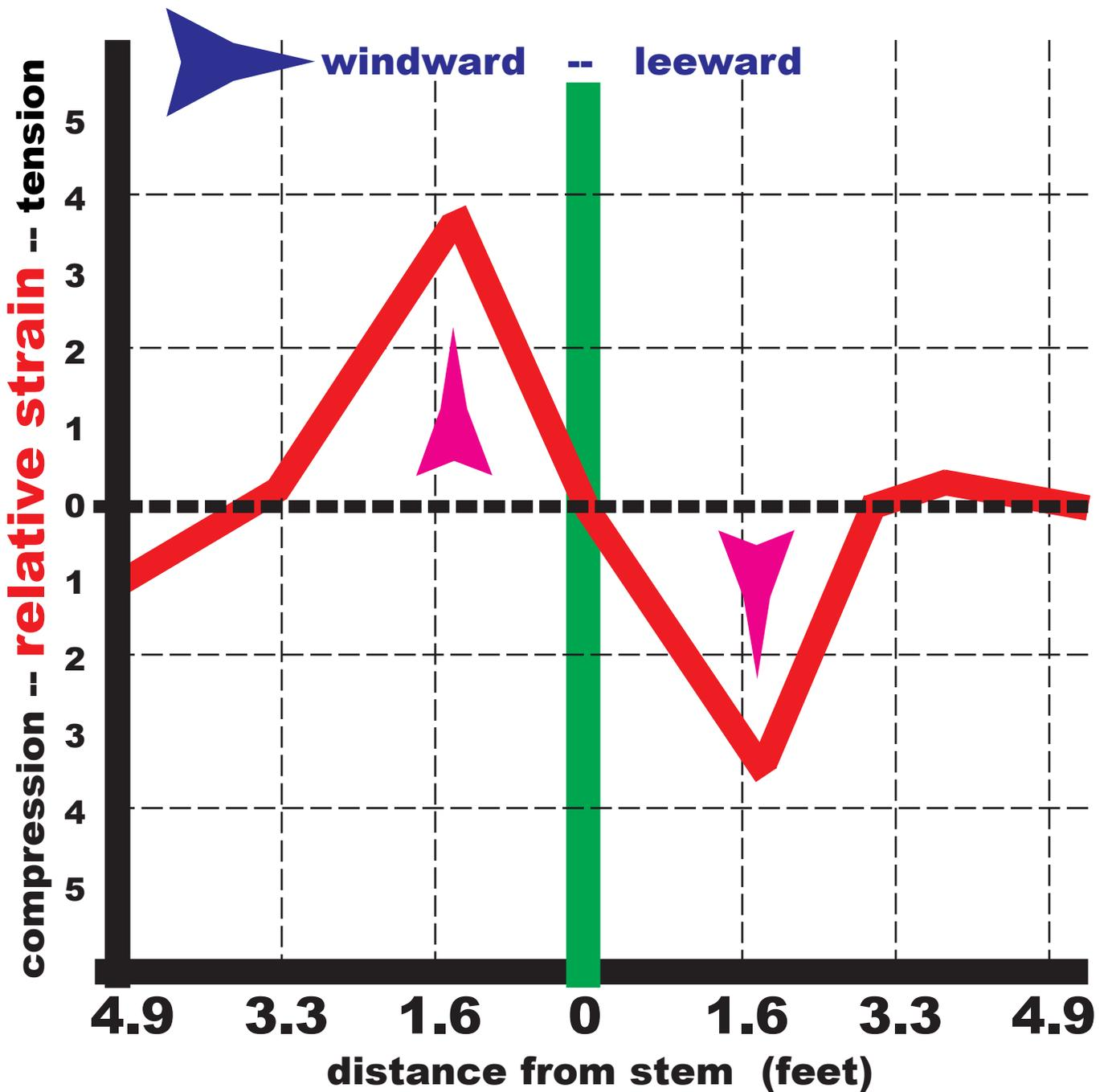
Figure 33: Root strain near tree base under lateral load.
