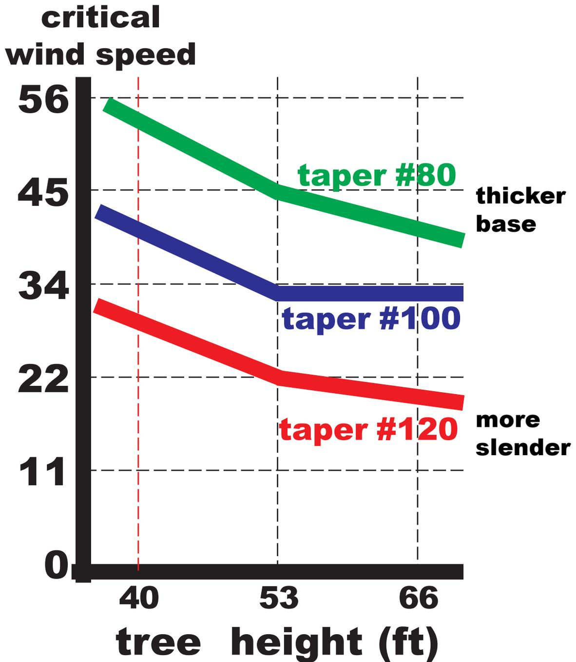
Figure 24: Critical wind speed (mph) measured at 33 feet in height for uprooting trees of different slenderness (height / dbh ratio or taper number).
