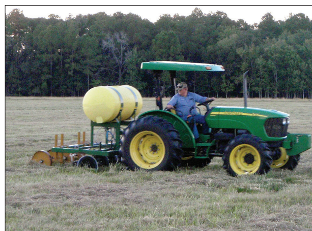
Figure 5. Tractor-pulled device for applying nematodes beneath the soil surface. (Lyle Buss, University of Florida)
