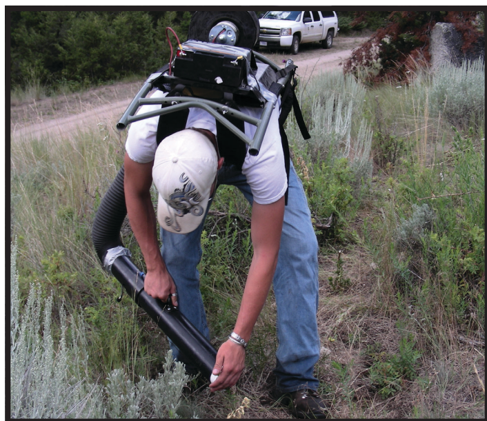
Figure 4. Motorized backpack vacuum sampler (Sharlene E. Sing, USDA FS RMRS)
